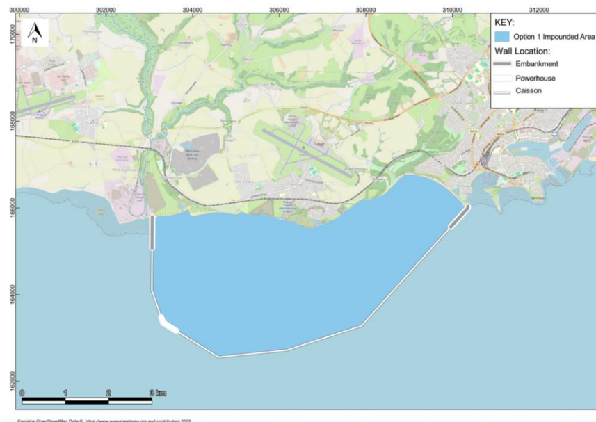
Figure 3: Plan on the proposed commercial demonstration lagoon in the Severn Estuary
