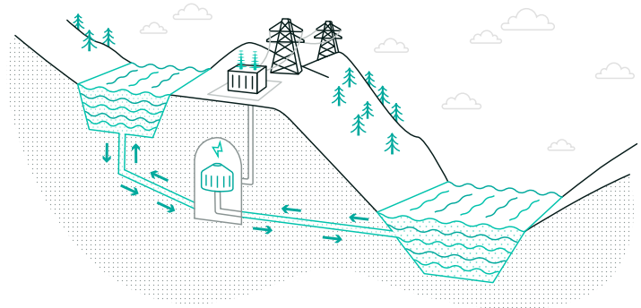
Upper and lower reservoir and the underground turbine hall.
