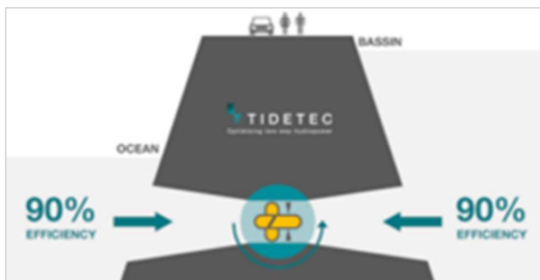
Figure 3-6 Rotating Turret Bulb Turbine Efficiency (Source: Tidetec)
