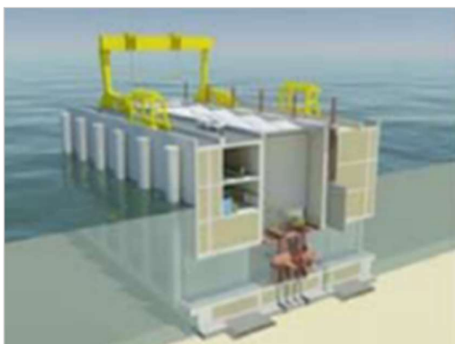
Figure 3-8 VLH Turbine and Caisson (Source: Atkins/Rolls-Royce)
